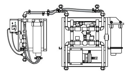
The Model 6979 Brominating System was designed to treat water generated by the ship's water makers as well as recirculate and treat the water in the ship's two water storage tanks.
