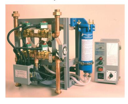
The electrical control panel can be mounted remotely, providing an extremely user-friendly installation. For example, the brominator/pump assembly can be mounted in a less accessible bilge area, while the control panel can be conveniently located in a stateroom or passageway.
